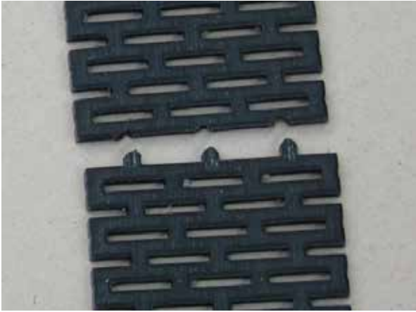
Figure 9. Typical orthogonal breakage
