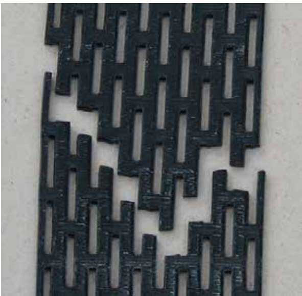
Figure 10. Typical parallel sample breakage
