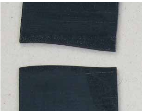
Figure 11. Typical plain sample breakage
