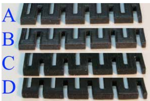
Figure 5. Outcome of four different print directions on parallel patterned pieces
